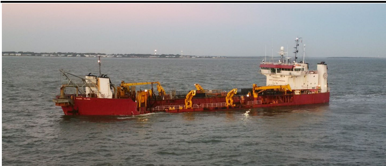
Figure 4: Hopper dredge Padre Island (owned/operated by Great Lakes Dredge & Dock) actively dredging with drag head deployed and sailing low in the water while loaded with material
