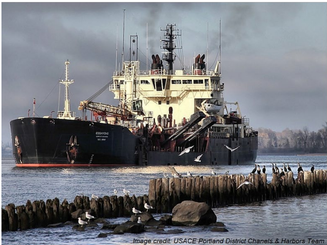
Figure 6: Top panel: Dredge Essayons sailing unloaded, note red section of hull visible above waterline. Bottom panel: Dredge Essayons sailing loaded, drafting 12–14 feet lower in the water with very little red section of hull visible above waterline.
