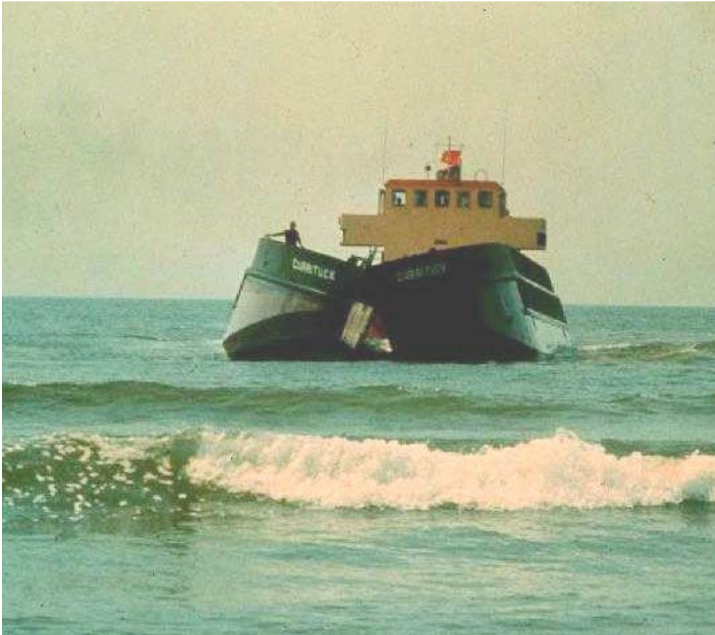
Figure 16: Dredge Currituck splitting open the hull to place material in the nearshore environment (Photo from EM 1110-2-5025)
