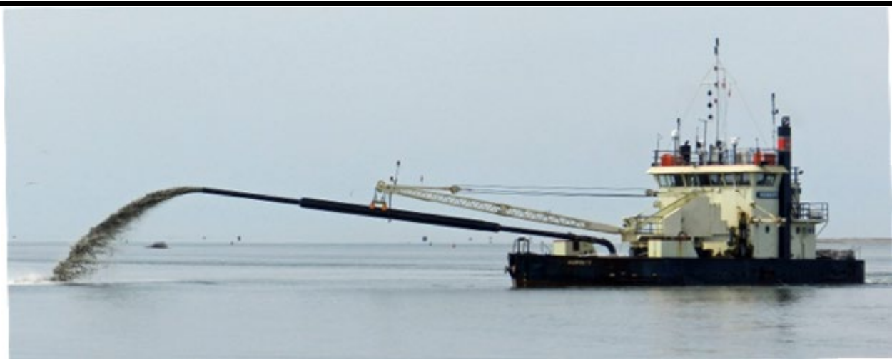
Figure 13. The USACE sidecasting dredge Merritt can work in locations too shallow for hopper dredges and too rough for pipeline dredges
