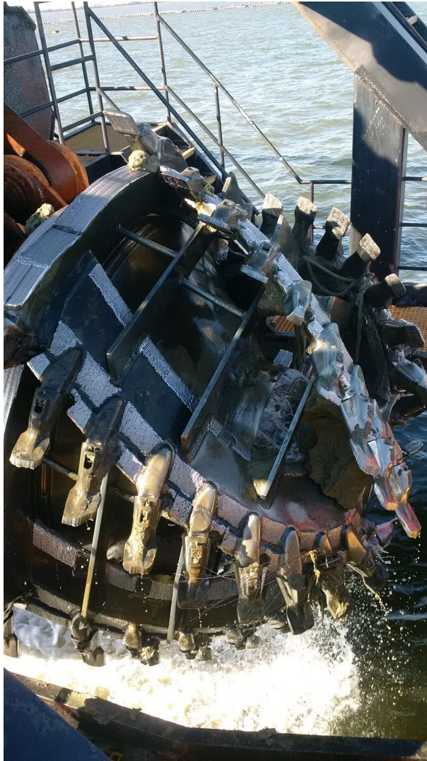
Figure 10: Close-up view of pipeline cutterhead showing interchangeable cutting teeth, which should be securely fastened before use. Debris can be caught in the cutterhead and needs to be cleared periodically. Debris often includes tires and wires.
