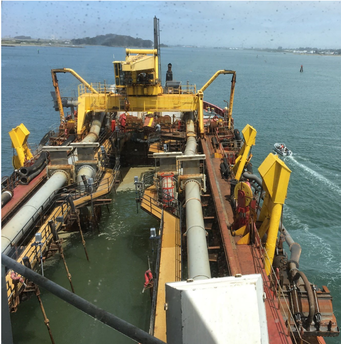
Figure 5: View from the bridge of a hopper dredge Terrapin Island (owned/operated by Great Lakes Dredge & Dock), looking down into the hopper while it is filled with slurry material
