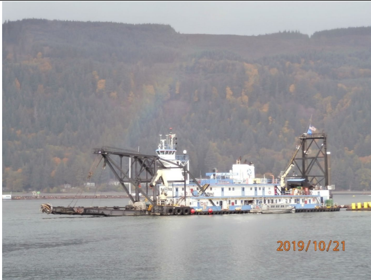
Figure 8: Port of Portland owned/operated Dredge Oregon (pipeline cutterhead dredge) operating on the Columbia River. The cutterhead is suspended above the water on the left side of the photo, the discharge pipeline is coming off the back of the dredge to the right. (Photo from Portland District)
