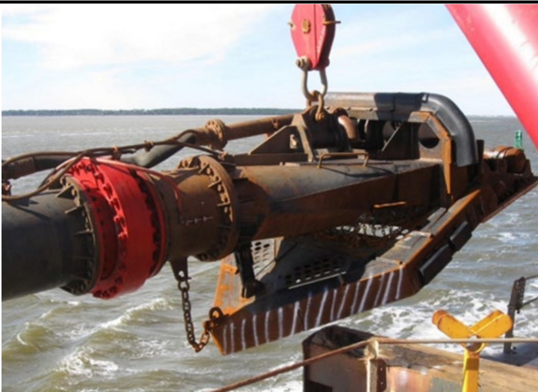
Figure 24: Hopper drag arm. White diagonal paint stripes are part of the paint test. The paint test is a quality control check to validate the ability of the TED to embed in the seafloor. The paint will wear off from abrasion if the TED is embedding properly in the seafloor.
